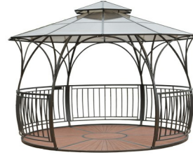
YG-G709C IRON GAZEBO WITH FLOOR Ø430*H300CM IRON FRAME+PC SHEET+PLASTIC FLOOR IRON COLUMN: 40X40X1.0MM
