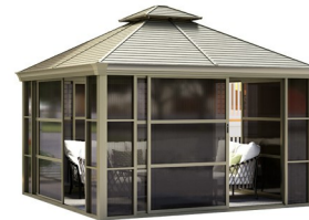
YG-G3636B ALUMINUM HOUSE GAZEBO W360*L360*H315CM ALU FRAME+PC SHEET+ GALVANIZED STEEL ROOF ALU COLUMN: 81X81X1.2MM
